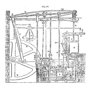
Watt's governor embedded on the reciprocating engine and connected to the flywheel and throttle valve. Noticeably, the boiler is not shown here. From John Bourne, <u>A Catechism of the Steam Engine</u>, 1854 at www.gutenberg.org/files/10998/10998-h/10998-h.htm.
